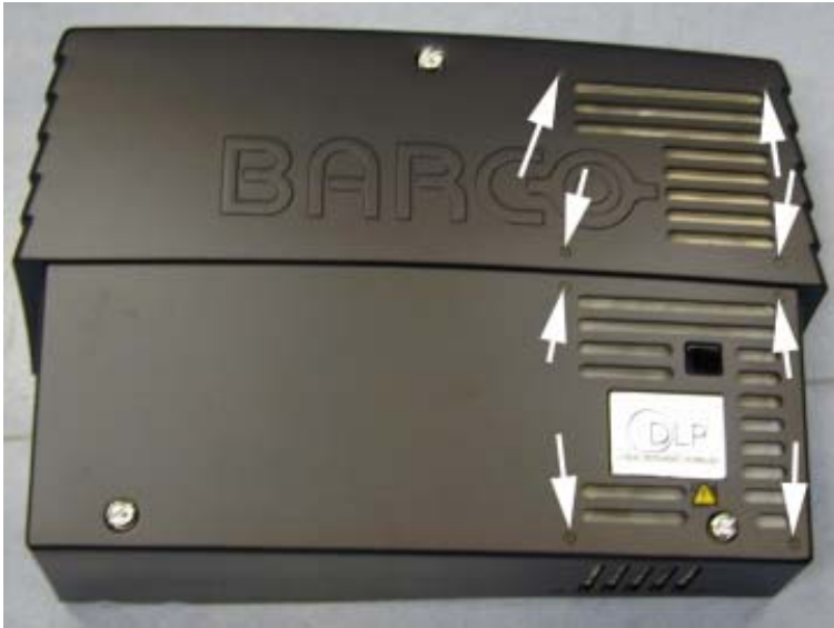
Image B-7 Dust filter removal
